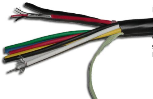
Kramer's BCP-6X2T is a unique plenum rated multi-conductor cable that supports a wide variety of signals used in typical professional AV systems. It contains six high-resolution mini coaxes and two 22 gauge shielded pairs in a remarkably small and lightweight profile
